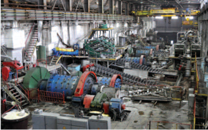
Figure 19: (left) the staged rod and mill, and spiral classifier at the Vostok-II mine, Russia (Schmidt 2012); (top) grinded tungsten ore stock ( Tungsten ore beneficiation process in Russia )
