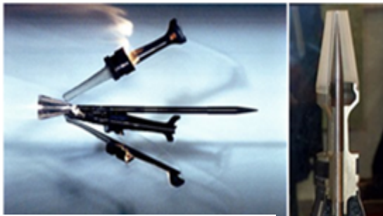
Figure 1: Kinetic Energy Penetrators; hard, dense and tough materials are required to transfer the maximum kinetic energy to a target. The rod-shaped penetrator and its carrier are illustrated in these pictures. Differently sized and shaped weapons are used for different purposes (Tanque Argentino (TAM) 2013)
