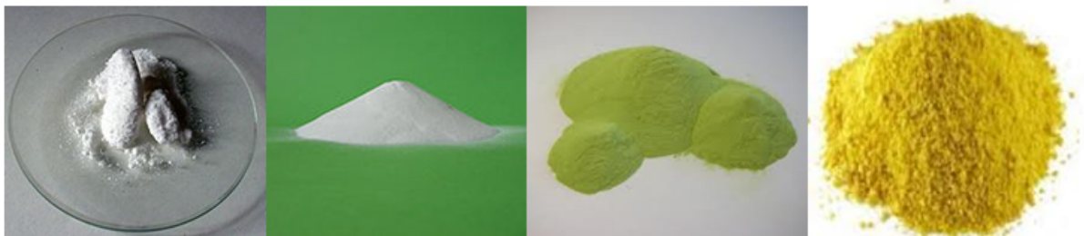
Figure 42: Sodium tungstate ( \text{Na}_2\text{WO}_4 \cdot 2\text{H}_2\text{O} ), ammonium paratungstate ( (\text{NH}_4)_{10}(\text{W}_{12}\text{O}_{41}) \cdot 5\text{H}_2\text{O} ), tungsten oxide ( \text{WO}_3 ) and tungstic acid ( \text{H}_2\text{WO}_4 ) are the main available tungsten compounds ( Sodium Tungstate 2014), ( Ammonium Paratungstate 2014), ( Tungsten Oxide ), (Stanovsky); they generally have colored nature making them interesting for being used as pigments.
