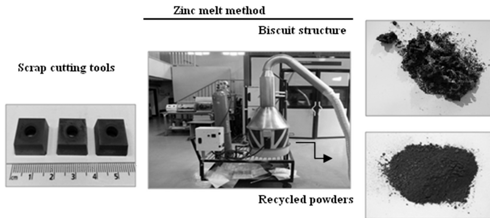
Figure 70: Tungsten recovery from cemented carbide via ZMM (Altuncu et al. 2013).
