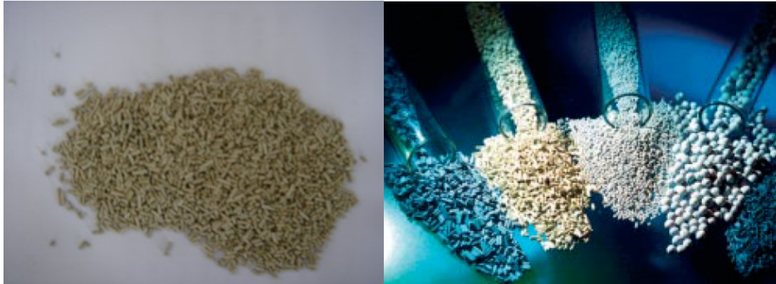
Figure 51: (Left) catalysts for hydrocracking process ( Hydrocracking catalysts ), and (Right) catalysts for HDS/HDN/HAD processes ( 17th Annual General Meeting 2004 ) the total formula for a HDS reaction is: C_xH_yS + 2H_2 \rightarrow C_xH_{(y+2)} + H_2S
