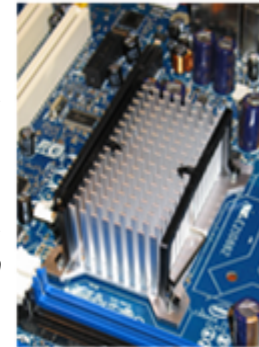
Figure 2: Heat Sinks in integrated systems require excellent heat conductivity as well as adequate dimensional stability. The mechanism of such cooling system is schematically shown (Intel GMA X3000 2014).
