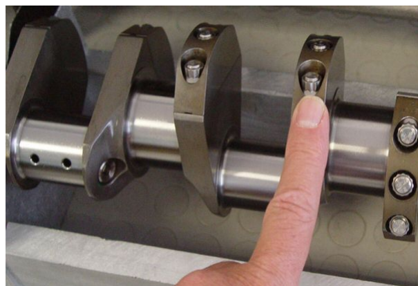
Figure 39: Crankshaft equipped with balance-weights of THAs ( Contemporary Crankshaft Design ).
