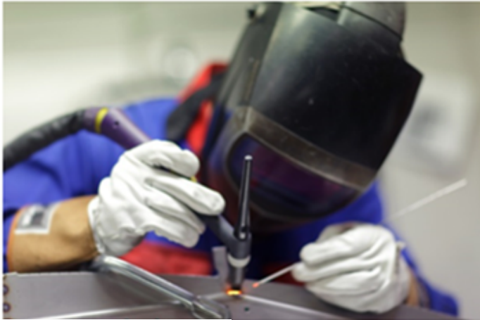
Figure 5: High melting temperature, low vapor pressure, low electrical resistivity and superior mechanical properties at elevated temperatures ensure the adequate performance of tungsten compounds as welding tips ( TIG Welding 2014 ).
