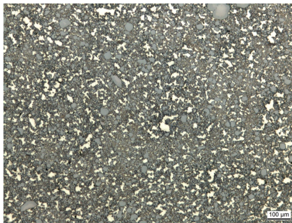
Figure 22: A common microstructure of hard metals ( WC Ag switch contacts for medium and low voltage ); this important family of metallic composites in which hard carbides powders are sintered in a matrix of tough metals. Such microstructure results in high strength as well as sufficient toughness.
