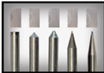
Figure 5: High melting temperature, low vapor pressure, low electrical resistivity and superior mechanical properties at elevated temperatures ensure the adequate performance of tungsten compounds as welding tips ( TIG Welding 2014 ).
